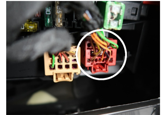
Red connector below fusebox (Always seen from wireside)
