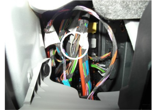
Ignition can alternative be found: Ignition switch, black 6-pin connector, pin 2, Black wire.
